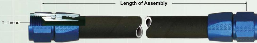
Hydrasearch AN-6270 low pressure hose assemblies can be used as flexible connections on low pressure or vacuum systems such as aircraft instrument systems (See SAE-AIR797). It is especially suited for low pressure hydraulic fluids, engine oils, fuels, and coolant fluids. Hydrasearch low pressure hose is used for applications with operating pressures to 250 psi, and having a temperature range of -67°F to +158°F.
