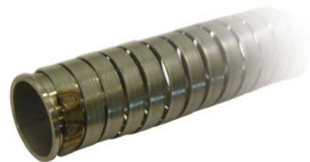
Used to prevent damage to assemblies subject to mishandling, high vacuum, or tight bend installations. Made of flat helically wound type 302 stainless steel.
